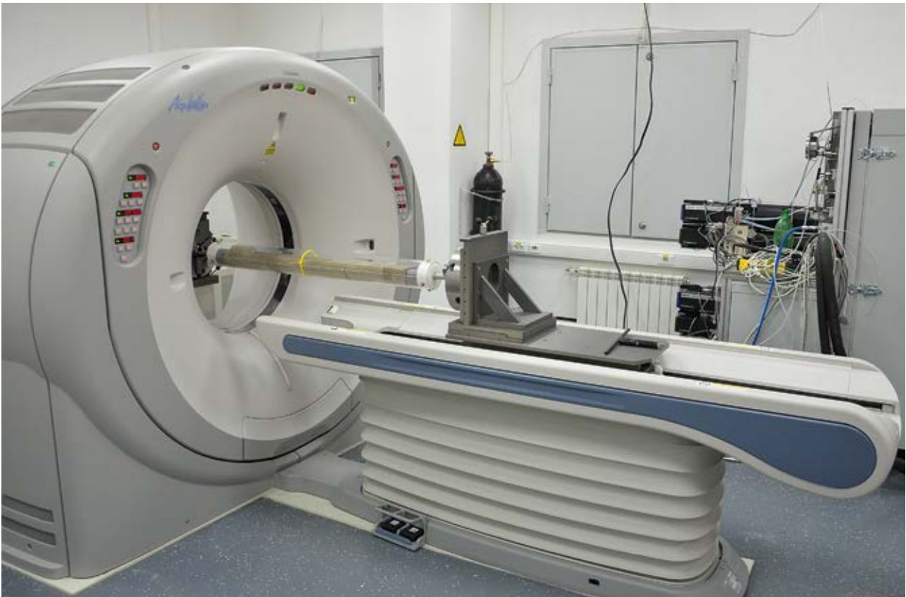
The tomograph with the filtration unit
