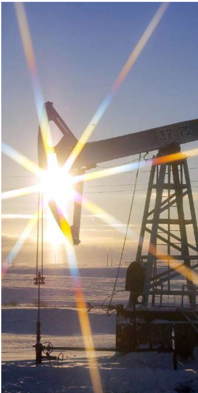
Sucker-rod pump at one of Udmurtneft's fields
